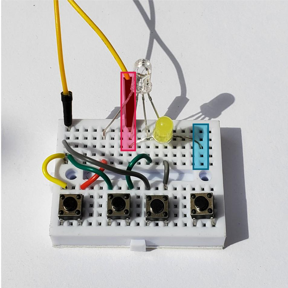
Attach your final long wire to the final open hole in the upper left row. Then attach that wire to the upper left of the final button. The last wire should attach from the upper right of the button to the free prong of the single-light LED. **Your circuit should be functioning at this point!** If the single-light LED doesn't light up, you can try switching the prongs of the LED around.
