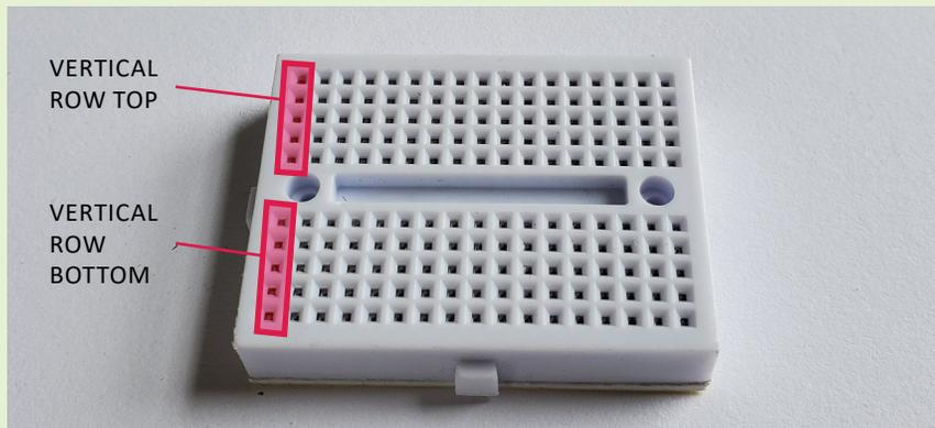
This means when these instructions say to “connect the left prong of this LED” to a wire, you can put the wire into any of the holes in the vertical row where the LED is positioned.
